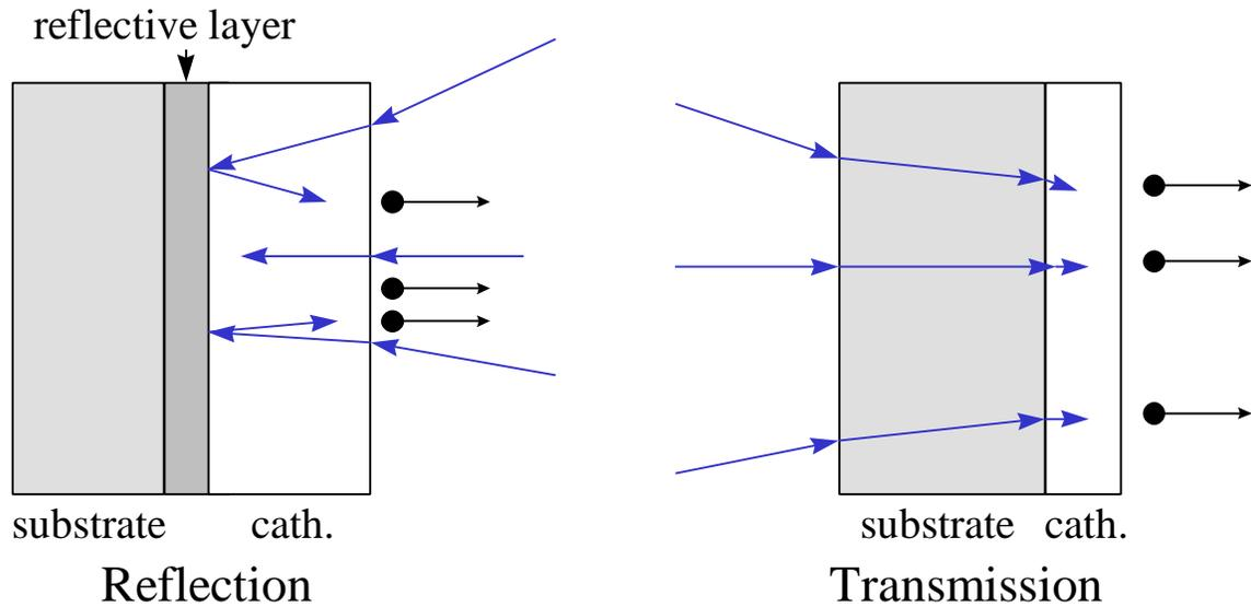
**Figure 1. Photocathode configurations (after Johnson<sup>3</sup>).**
